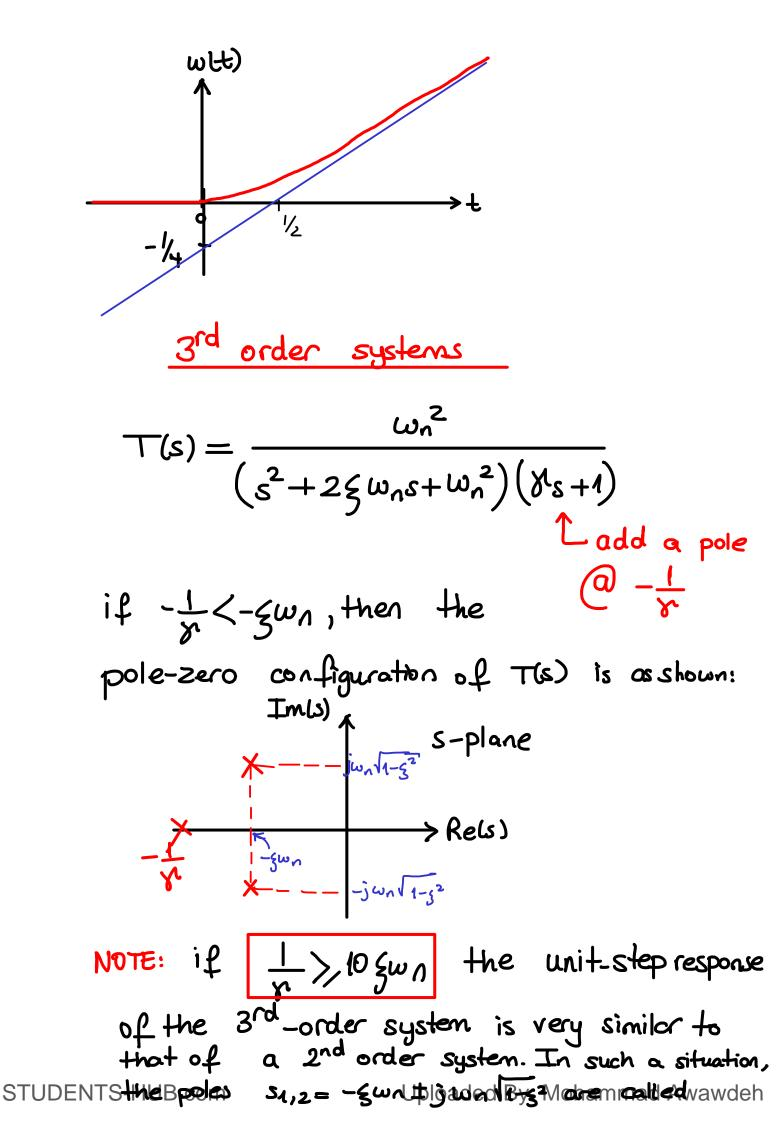
"dominant poles" and the pole at  $-\frac{1}{8}$  is called an insignificant pole. If  $\frac{1}{2}$  losur then the response of the 3<sup>rd</sup> order system is significantly different from that of the 2<sup>rd</sup> order system. Then we can't use the expressions derived for Ts, Tp, Tr, etc.
