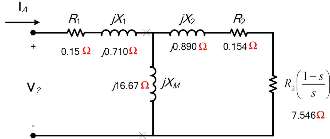
The phase voltage must be derated by 5/6, so  $V_\phi = 212.5 \text{ V}$ .
