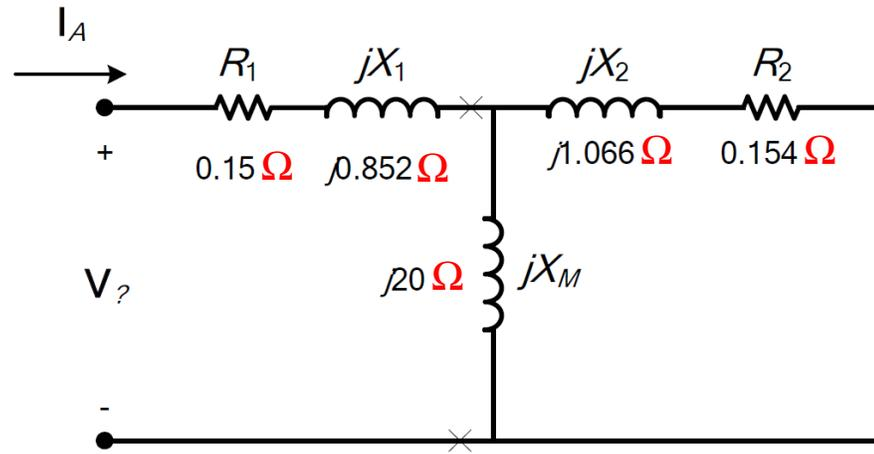
The easiest way to find the line current (or armature current) is to get the equivalent impedance  $Z_F$  of the rotor circuit in parallel with  $jX_M$ , and then calculate the current as the phase voltage divided by the sum of the series impedances, as shown below.
