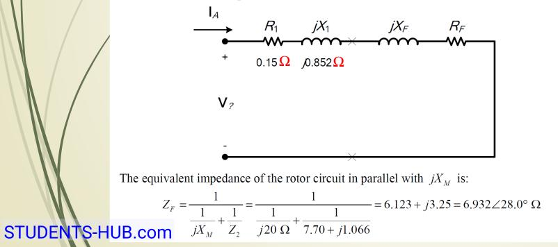
The phase voltage is  $460/\sqrt{3} = 266$  V, so line current  $I_L$  is
