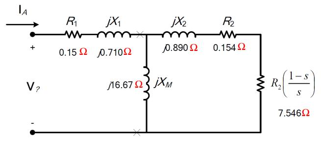
The phase voltage must be derated by 5/6, so  $V_{\phi} = 212.5$  V.
