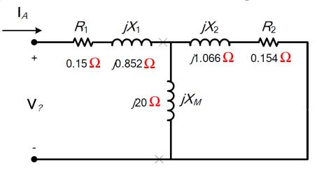
The easiest way to find the line current (or armature current) is to get the equivalent impedance  $Z_F$  of the rotor circuit in parallel with  $jX_M$ , and then calculate the current as the phase voltage divided by the sum of the series impedances, as shown below.
