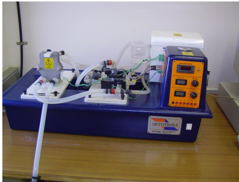
Figure 1 shows the experimental heat exchanger.
