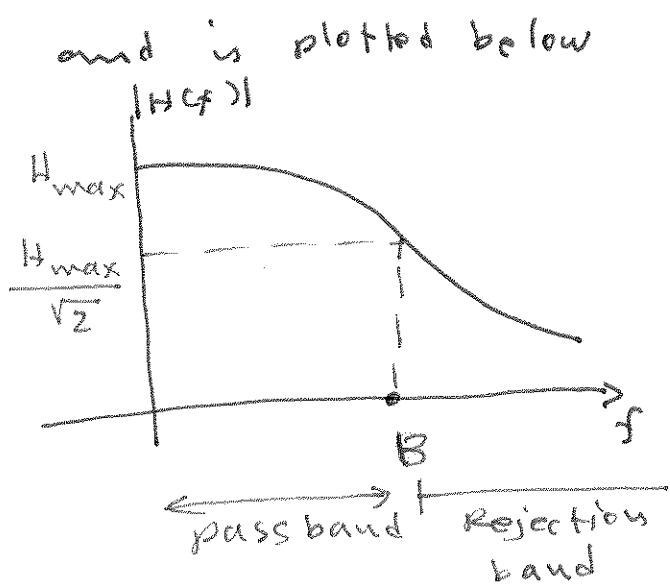
Note that  $20 \log \frac{|H(f_c)|}{H_{max}} = 20 \log \frac{1/\sqrt{2}}{1} = -20 \log \sqrt{2} = -3 \text{ dB}$
