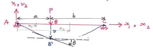
If instead the elastic curve is expressed in terms of the coordinaks  $0 \leqslant x_1 \leqslant a$  and  $0 \leqslant x_2 \leqslant b$ , as shown below, then the continuous of slope and deflection at B requires  $\theta_1(x_1=a) = -\theta_2(x_2=b)$  sign is necessary to match the slopes at B since  $x_1$  extends Consequently,  $\theta_1$  is positive counterclock wise, and  $\theta_2$  is positive to the left.
