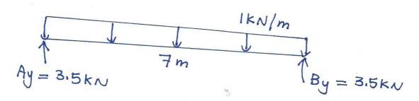
b) Write the internal moment as a function of x:
