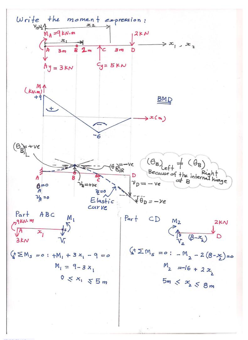
$$\frac{P_{art} \quad AB:}{d^{2}v_{AB}} = q - 3 \times, \qquad \sum_{i=1}^{\infty} \frac{1}{dx_{i}} = q_{x_{i}} - \frac{3}{2}x_{i}^{2} + C_{i}$$
