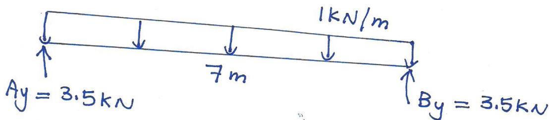
b) Write the internal moment as a function of  $x$ :
