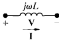
Figure 7.3: The frequency-domain equivalent circuit for an inductor
