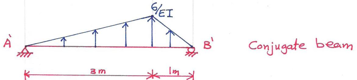
Determine the reactions at points A' and B' on the conjugate beam.
