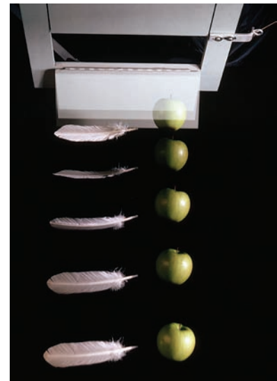
Fig. 2-10 A feather and an apple free fall in vacuum at the same magnitude of acceleration g . The acceleration increases the distance between successive images. In the absence of air, the feather and apple fall together. (Jim Sugar/Corbis Images)
