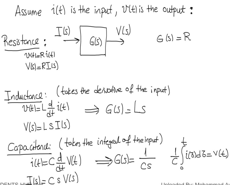
In sinusoidal steady state, Resistance, Inductore,
