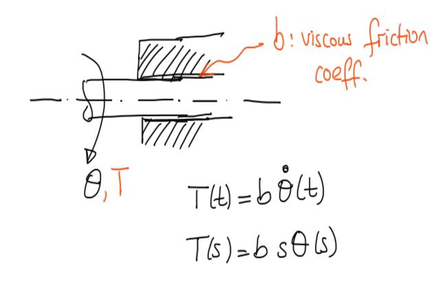
EX: (Torsional pendulum system) J: inertia Egn of Motion 000  $T\hat{\Theta} = T(t) - T_k(t) - T_b(t)$ 2, TH), O(L)  $T\ddot{\theta} = T(t) - k\theta - b\dot{\theta}$  $\int \int \Theta(0) = \dot{\Theta}(0) = 0$  $Js^2\Theta(s) = T(s) - k\Theta(s) - bs\Theta(s)$  $=\frac{1}{Js^2+bs+k}$  2<sup>nd</sup> order f.f.
