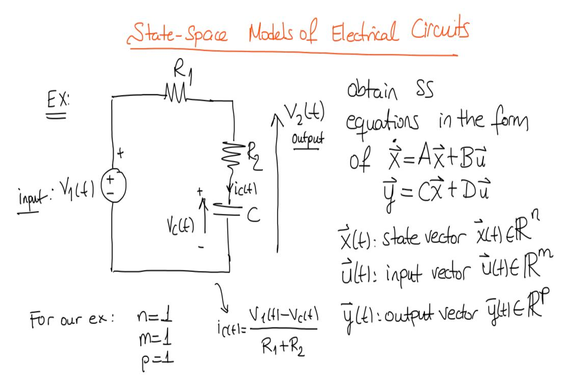
$$C \frac{d}{dt} V_{C}(t) = i_{C}(t)$$
