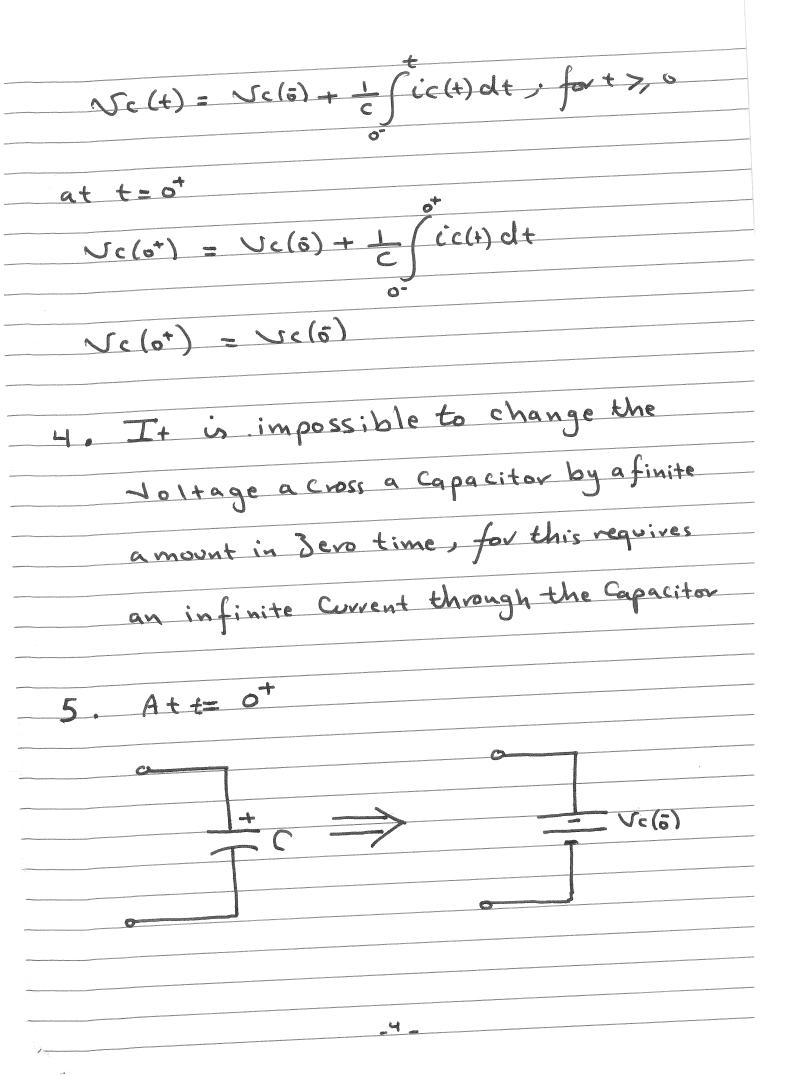
A capacitor is therefore an open circuit to dc
