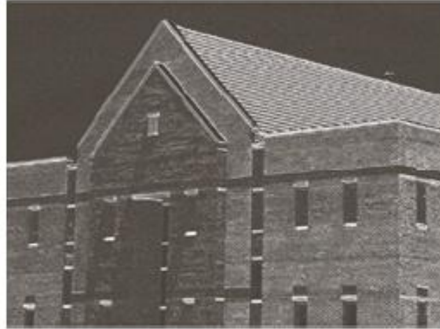
Gx computed using Sobel Operator
