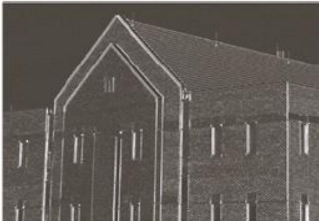
Gy computed using Sobel Operator
