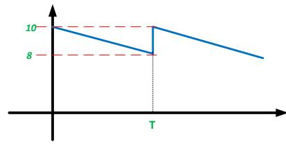
$$\begin{aligned}V_{O,DC} &= V_{O,AVG} = \frac{1}{T} \int_0^T V_O(t) dt \\&= \frac{1}{T} (\text{Area}) \\&= \frac{1}{T} \left( 8T + \frac{2T}{2} \right) = 9 \text{ V}\end{aligned}$$
