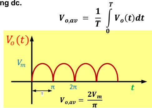
$$V_{i,av} = \frac{1}{T} \int_0^T V_i(t) dt = 0$$
