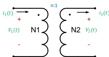
$$\frac{V_2(t)}{V_1(t)} = \frac{N_2}{N_1}$$
