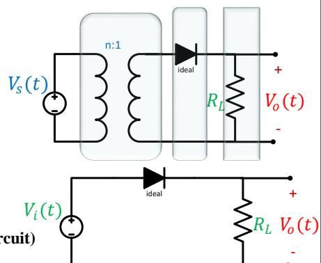
B) when  $V_i(t) < 0$ , Diode is off (open circuit)
