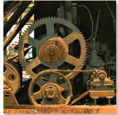
The gears used in the operation of a crane all rotate about fixed axes. Engineers must be able to relate their angular motions in order to properly design this gear system. (© R.C. Hibbeler)
