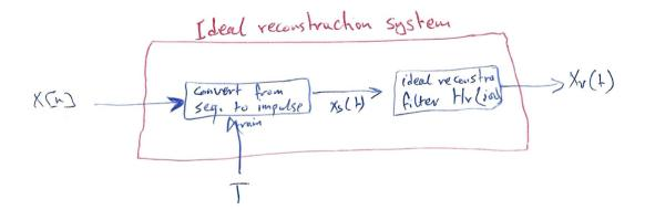
\* Discrete-time processing of Continuous-time Signals
