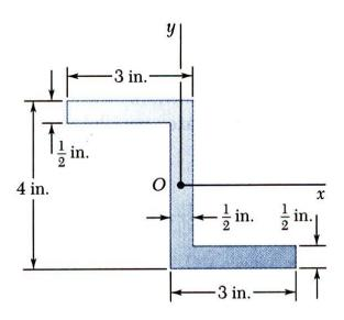
For the section shown, the moments of inertia with respect to the x and y axes are  $I_x = 10.38$  in<sup>4</sup> and  $I_y = 6.97$  in<sup>4</sup>.
