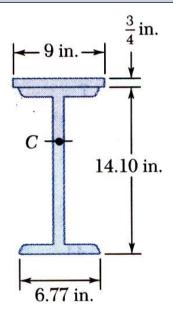
The strength of a W14x38 rolled steel beam is increased by attaching a plate to its upper flange.
