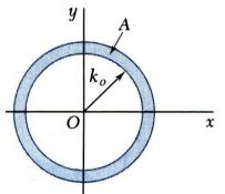
• Consider area A with moment of inertia  $I_x$ . Imagine that the area is concentrated in a thin strip parallel to the x axis with equivalent  $I_x$ .
