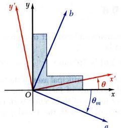
• The moments and product of inertia for an area are plotted as shown and used to construct *Mohr's circle*,
