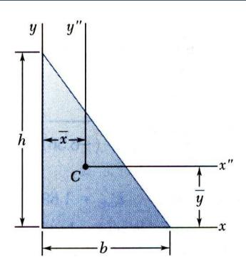
• Apply the parallel axis theorem to evaluate the product of inertia with respect to the centroidal axes.
