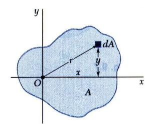
• The *polar moment of inertia* is an important parameter in problems involving torsion of cylindrical shafts and rotations of slabs.
