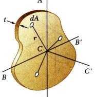
• For the axis CC' which is perpendicular to the plate,
