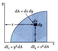
• Second moments or moments of inertia of an area with respect to the x and y axes,
