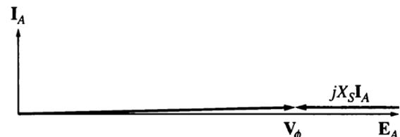
The above phasor diagram of a Synchronous Condenser at no load is similar to the phasor diagram of a passive capacitor, where  $\overline{I}_A$  leads  $\overline{V}_\phi$ ; the **motor looks like a large capacitor**.
