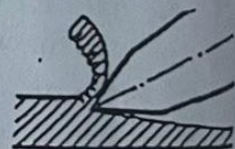
inclination too great, the chisel will slide off the work piece.
