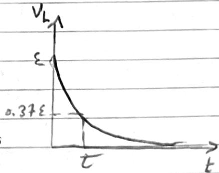
$\tau$ : a measure of how fast the current rises in the circuit
