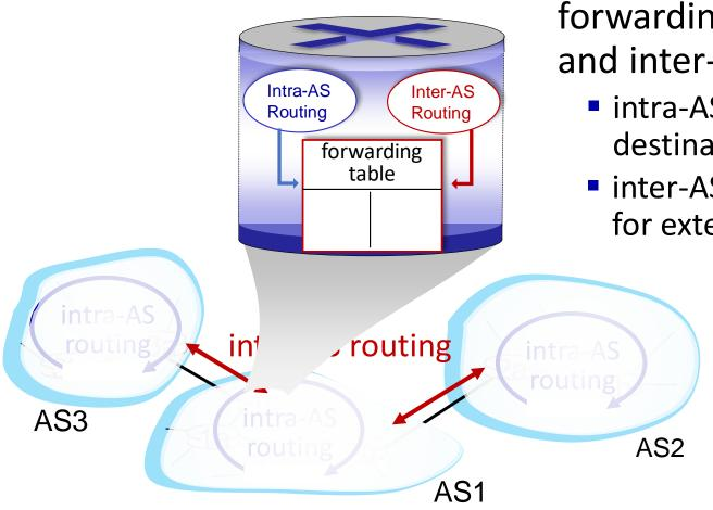
forwarding table configured by intraand inter-AS routing algorithms
