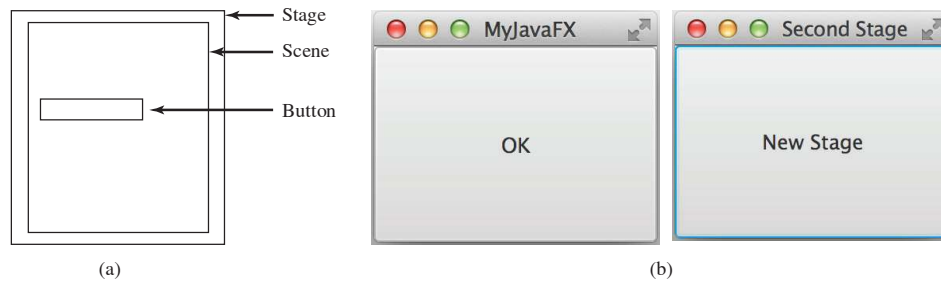
FIGURE 14.2 (a) Stage is a window for displaying a scene that contains nodes. (b) Multiple stages can be displayed in a JavaFX program.
