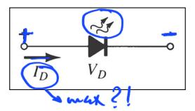
The forward bias voltage is usually in the range of 2 V to 3 V.
