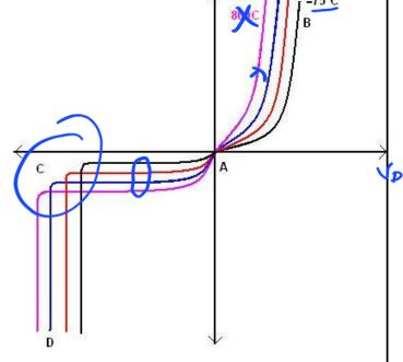
Germanium diodes are more sensitive to temperature variations than silicon or gallium arsenide diodes.
