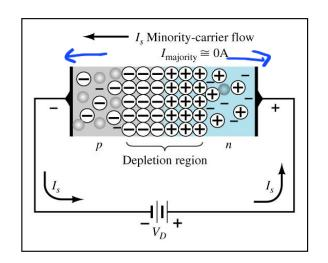
The holes in the *p*-type material are attracted toward the negative terminal of the voltage source.
