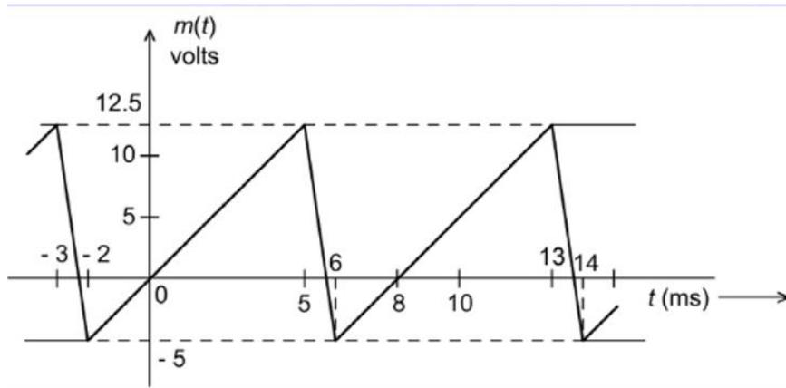
If  $(f_i)_{\max} - (f_i)_{\min}$  is to be 100 kHz show that  $k_p = 10\pi$  rad/volt.
