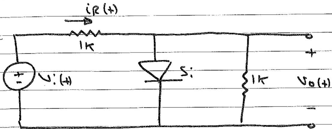
$V_i(t) = 10 \sin \omega t \text{ V}$
