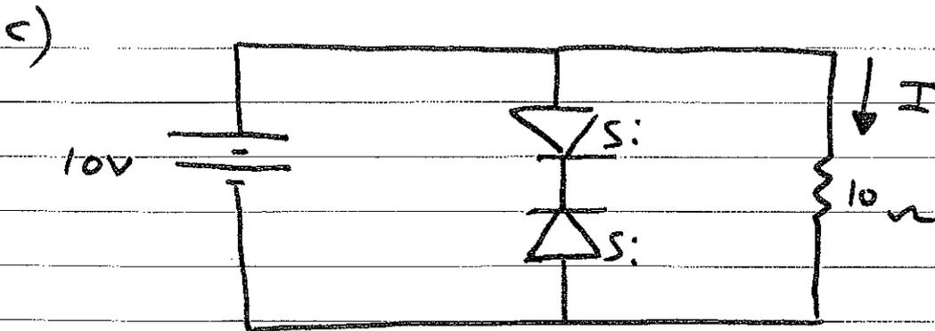
Both diodes are OFF, replace them with open circuit
