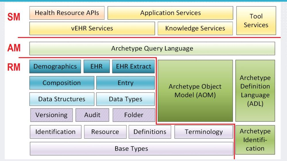
Dependency between components is from the bottom to top All components use data types & data structures from RM STUDENTS-HUB.com
