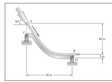
The nozzle discharges water at the rate of 340 gal/min. Knowing the velocity of the water at both A and B has a magnitude of 65 ft/s and neglecting the weight of the vane, determine the components of the reactions at C and D. (1 ft<sup>3</sup> = 7.48 gallons)
