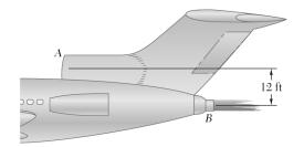
The jet engine shown scoops in air at A at a rate of 200 lb/s and discharges it at B with a velocity of 2000 ft/s relative to the airplane. Determine the magnitude and line of action of the propulsive thrust developed by the engine when the speed of the airplane is (a) 300 mi/h, (b) 600 mi/h.
