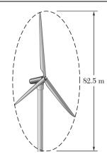
A wind turbine-generator system having a diameter of 82.5 m produces 1.5 MW at a wind speed of 12 m/s. Determine the diameter of blade necessary to produce 10 MW of power assuming the efficiency is the same for both designs and  $\rho = 1.21 \text{ kg/m}^3$  for air.
