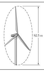
The wind turbine-generator shown has an output-power rating of 1.5 MW for a wind speed of 36 km/h. For the given wind speed, determine (a) the kinetic energy of the air particles entering the 82.5-m-diameter circle per second, (b) the efficiency of this energy conversion system. Assume  $\rho = 1.21 \text{ kg/m}^3$  for air.
