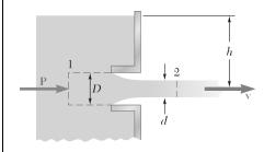
A circular reentrant orifice (also called Borda's mouthpiece) of diameter D is placed at a depth h below the surface of a tank. Knowing that the speed of the issuing stream is  $v = \sqrt{2gh}$  and assuming that the speed of approach  $v_1$  is zero, show that the diameter of the stream is  $d = D/\sqrt{2}$ . (*Hint*: Consider the section of water indicated, and note that P is equal to the pressure at a depth h multiplied by the area of the orifice).
