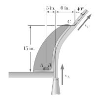
The nozzle shown discharges water at the rate of 200 gal/min. Knowing that at both B and C the stream of water moves with a velocity of magnitude 100 ft/s, and neglecting the weight of the vane, determine the force-couple system which must be applied at A to hold the vane in place (1 ft<sup>3</sup> = 7.48 gal).
