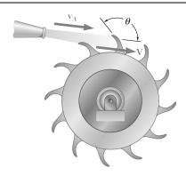
In a Pelton-wheel turbine, a stream of water is deflected by a series of blades so that the rate at which water is deflected by the blades is equal to the rate at which water issues from the nozzle  $(\Delta m/\Delta t = A\rho v_A)$ . Using the same notation as in Sample Problem 14.7, (a) determine the velocity  $\mathbf{V}$  of the blades for which maximum power is developed, (b) derive an expression for the maximum power, (c) derive an expression for the mechanical efficiency.
