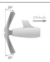
In order to shorten the distance required for landing, a jet airplane is equipped with movable vanes, which partially reverse the direction of the air discharged by each of its engines. Each engine scoops in the air at a rate of 120 kg/s and discharges it with a velocity of 600 m/s relative to the engine. At an instant when the speed of the airplane is 270 km/h, determine the reverse thrust provided by each of the engines.
