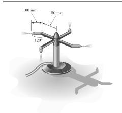
A garden sprinkler has four rotating arms, each of which consists of two horizontal straight sections of pipe forming an angle of  $120^{\circ}$  with each other. Each arm discharges water at a rate of 20 L/min with a velocity of 18 m/s relative to the arm. Knowing that the friction between the moving and stationary parts of the sprinkler is equivalent to a couple of magnitude  $M = 0.375 \,\mathrm{N} \cdot \mathrm{m}$ , determine the constant rate at which the sprinkler rotates.
