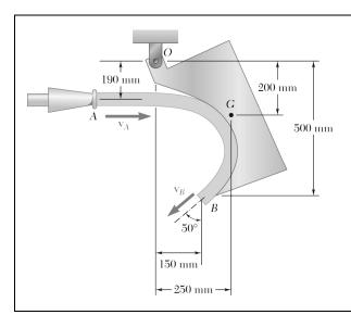
A high speed jet of air issues from the nozzle A with a velocity of  $\mathbf{v}_A$  and mass flow rate of 0.36 kg/s. The air impinges on a vane causing it to rotate to the position shown. The vane has a mass of 6-kg. Knowing that the magnitude of the air velocity is equal at A and B determine (a) the magnitude of the velocity at A, (b) the components of the reactions at O.
