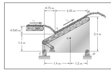
Coal is being discharged from a first conveyor belt at the rate of 120 kg/s. It is received at A by a second belt which discharges it again at B. Knowing that  $v_1 = 3$  m/s and  $v_2 = 4.25$  m/s and that the second belt assembly and the coal it supports have a total mass of 472 kg, determine the components of the reactions at C and D.
