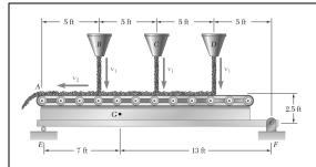
Sand falls from three hoppers onto a conveyor belt at a rate of 90 lb/s for each hopper. The sand hits the belt with a vertical velocity  $v_1 = 10$  ft/s and is discharged at A with a horizontal velocity  $v_2 = 13$  ft/s. Knowing that the combined mass of the beam, belt system, and the sand it supports is 1300 lb with a mass center at G, determine the reaction at E.
