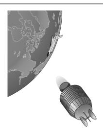
A communication satellite weighing 10,000 lb, including fuel, has been ejected from a space shuttle describing a low circular orbit around the earth. After the satellite has slowly drifted to a safe distance from the shuttle, its engine is fired to increase its velocity by 8000 ft/s as a first step to its transfer to a geosynchronous orbit. Knowing that the fuel is ejected with a relative velocity of 13,750 ft/s, determine the weight of fuel consumed in this maneuver.
