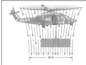
The helicopter shown can produce a maximum downward air speed of 80 ft/s in a 30-ft-diameter slipstream. Knowing that the weight of the helicopter and its crew is 3500 lb and assuming  $\gamma = 0.076 \text{ lb/ft}^3$  for air, determine the maximum load that the helicopter can lift while hovering in midair.
