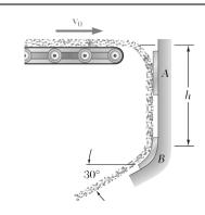
A mass q of sand is discharged per unit time from a conveyor belt moving with a velocity  $\mathbf{v}_0$ . The sand is deflected by a plate at A so that it falls in a vertical stream. After falling a distance h the sand is again deflected by a curved plate at B. Neglecting the friction between the sand and the plates, determine the force required to hold in the position shown (a) plate A, (b) plate B.
