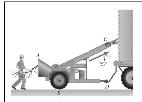
Tree limbs and branches are being fed at A at the rate of 5 kg/s into a shredder which spews the resulting wood chips at C with a velocity of 20 m/s. Determine the horizontal component of the force exerted by the shredder on the truck hitch at D.
