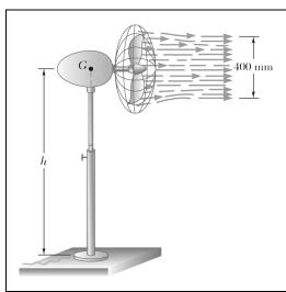
A floor fan designed to deliver air at a maximum velocity of 6 m/s in a 400-mm-diameter slipstream is supported by a 200-mm-diameter circular base plate. Knowing that the total weight of the assembly is 60 N and that its center of gravity is located directly above the center of the base plate, determine the maximum height h at which the fan may be operated if it is not to tip over. Assume  $\rho = 1.21 \, \text{kg/m}^3$  for air and neglect the approach velocity of the air.
