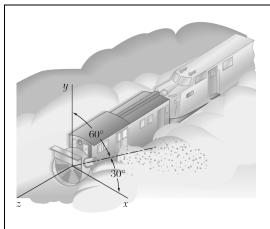
A rotary power plow is used to remove snow from a level section of railroad track. The plow car is placed ahead of an engine which propels it at a constant speed of 20 km/h. The plow car clears 160 Mg of snow per minute, projecting it in the direction shown with a velocity of 12 m/s relative to the plow car. Neglecting friction, determine (a) the force exerted by the engine on the plow car, (b) the lateral force exerted by the track on the plow.
