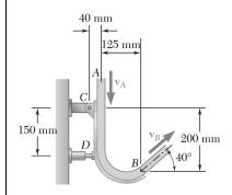
The stream of water shown flows at a rate of 550 liters/min and moves with a velocity of magnitude 18 m/s at both A and B. The vane is supported by a pin and bracket at C and by a load cell at D which can exert only a horizontal force. Neglecting the weight of the vane, determine the components of the reactions at C and D.
