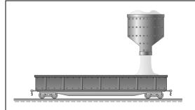
A railroad car of length L and mass  $m_0$  when empty is moving freely on a horizontal track while being loaded with sand from a stationary chute at a rate dm/dt = q. Knowing that the car was approaching the chute at a speed  $v_0$ , determine (a) the mass of the car and its load after the car has cleared the chute, (b) the speed of the car at that time.
