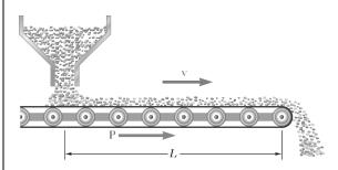
Gravel falls with practically zero velocity onto a conveyor belt at the constant rate q = dm/dt. (a) Determine the magnitude of the force **P** required to maintain a constant belt speed v. (b) Show that the kinetic energy acquired by the gravel in a given time interval is equal to half the work done in that interval by the force **P**. Explain what happens to the other half of the work done by **P**.
