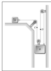
Slider block A moves to the left with a constant velocity of 6 m/s. Determine (a) the velocity of block B, (b) the velocity of portion D of the cable, (c) the relative velocity of portion C of the cable with respect to portion D.
