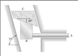
The assembly of rod A and wedge B starts from rest and moves to the right with a constant acceleration of 2 mm/s<sup>2</sup>. Determine (a) the acceleration of wedge C, (b) the velocity of wedge C when t = 10 s.
