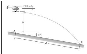
A helicopter is flying with a constant horizontal velocity of 180 km/h and is directly above Point A when a loose part begins to fall. The part lands 6.5 s later at Point B on an inclined surface. Determine (a) the distance d between Points A and B, (b) the initial height h.
