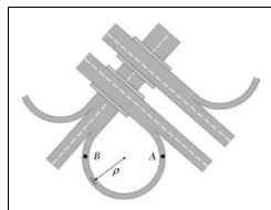
Determine the smallest radius that should be used for a highway if the normal component of the acceleration of a car traveling at 72 km/h is not to exceed  $0.8 \text{ m/s}^2$ .
