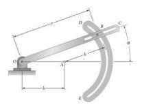
The pin at B is free to slide along the circular slot DE and along the rotating rod OC. Assuming that the rod OC rotates at a constant rate  $\theta$ , (a) show that the acceleration of pin B is of constant magnitude, (b) determine the direction of the acceleration of pin B.
