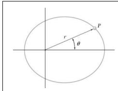
The path of particle P is the ellipse defined by the relations  $r = 2/(2 - \cos \pi t)$  and  $\theta = \pi t$ , where r is expressed in meters, t is in seconds, and  $\theta$  is in radians. Determine the velocity and the acceleration of the particle when (a) t = 0, (b) t = 0.5 s.
