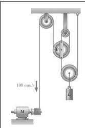
The motor M reels in the cable at a constant rate of 100 mm/s. Determine (a) the velocity of load L, (b) the velocity of pulley B with respect to load L.
