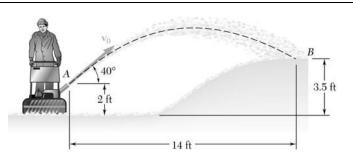
A homeowner uses a snowblower to clear his driveway. Knowing that the snow is discharged at an average angle of  $40^{\circ}$  with the horizontal, determine the initial velocity  $v_0$  of the snow.
