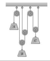
Block A starts from rest at t = 0 and moves downward with a constant acceleration of 6 in./s<sup>2</sup>. Knowing that block B moves up with a constant velocity of 3 in./s, determine (a) the time when the velocity of block C is zero, (b) the corresponding position of block C.
