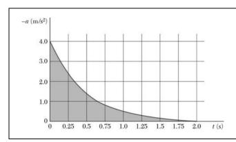
Two seconds are required to bring the piston rod of an air cylinder to rest; the acceleration record of the piston rod during the 2 s is as shown. Determine by approximate means (a) the initial velocity of the piston rod, (b) the distance traveled by the piston rod as it is brought to rest.
