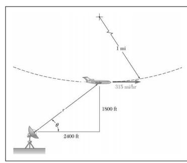
At the bottom of a loop in the vertical plane, an airplane has a horizontal velocity of 315 mi/h and is speeding up at a rate of 10 ft/s<sup>2</sup>. The radius of curvature of the loop is 1 mi. The plane is being tracked by radar at O. What are the recorded values of  $\dot{r}$ ,  $\ddot{r}$ ,  $\dot{\theta}$  and  $\ddot{\theta}$  for this instant?
