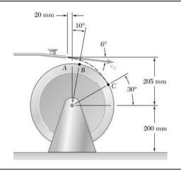
The nozzle at A discharges cooling water with an initial velocity  $\mathbf{v}_0$  at an angle of  $6^{\circ}$  with the horizontal onto a grinding wheel 350 mm in diameter. Determine the range of values of the initial velocity for which the water will land on the grinding wheel between Points B and C.
