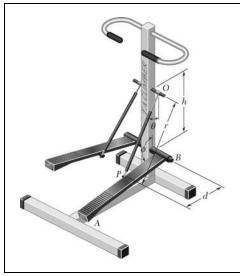
Show that  $\dot{r} = h\dot{\phi}\sin\theta$  knowing that at the instant shown, step AB of the step exerciser is rotating counterclockwise at a constant rate  $\dot{\phi}$ .
