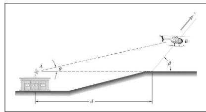
After taking off, a helicopter climbs in a straight line at a constant angle  $\beta$ . Its flight is tracked by radar from Point A. Determine the speed of the helicopter in terms of d,  $\beta$ ,  $\theta$ , and  $\dot{\theta}$ .
