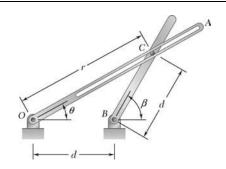
Pin C is attached to rod BC and slides freely in the slot of rod OA which rotates at the constant rate  $\omega$ . At the instant when  $\beta = 60^{\circ}$ , determine (a)  $\dot{r}$  and  $\dot{\theta}$ , (b)  $\ddot{r}$  and  $\ddot{\theta}$ . Express your answers in terms of d and  $\omega$ .
