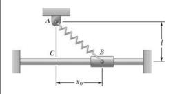
A spring AB is attached to a support at A and to a collar. The unstretched length of the spring is l. Knowing that the collar is released from rest at  $x = x_0$  and has an acceleration defined by the relation  $a = -100(x - lx/\sqrt{l^2 + x^2})$ , determine the velocity of the collar as it passes through Point C.
