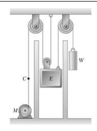
The elevator shown in the figure moves downward with a constant velocity of 4 m/s. Determine (a) the velocity of the cable C, (b) the velocity of the counterweight W, (c) the relative velocity of the cable C with respect to the elevator, (d) the relative velocity of the counterweight W with respect to the elevator.
