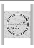
Pin P moves at a constant speed of 150 mm/s in a counterclockwise sense along a circular slot which has been milled in the slider block A shown. Knowing that the block moves downward at a constant speed 100 mm/s determine the velocity of pin P when (a)  $\theta = 30^{\circ}$ , (b)  $\theta = 120^{\circ}$ .
