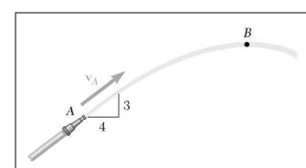
From measurements of a photograph, it has been found that as the stream of water shown left the nozzle at A, it had a radius of curvature of 25 m. Determine (a) the initial velocity  $\mathbf{v}_A$  of the stream, (b) the radius of curvature of the stream as it reaches its maximum height at B.
