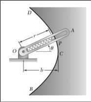
As rod OA rotates, pin P moves along the parabola BCD. Knowing that the equation of this parabola is  $r = 2b/(1 + \cos \theta)$  and that  $\theta = kt$ , determine the velocity and acceleration of P when (a)  $\theta = 0$ , (b)  $\theta = 90^{\circ}$ .
