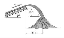
Sand is discharged at A from a conveyor belt and falls onto the top of a stockpile at B. Knowing that the conveyor belt forms an angle  $\alpha = 25^{\circ}$  with the horizontal, determine (a) the speed  $v_0$  of the belt, (b) the radius of curvature of the trajectory described by the sand at Point B.
