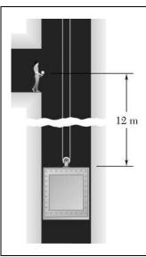
An elevator starts from rest and moves upward, accelerating at a rate of 1.2 m/s<sup>2</sup> until it reaches a speed of 7.8 m/s, which it then maintains. Two seconds after the elevator begins to move, a man standing 12 m above the initial position of the top of the elevator throws a ball upward with an initial velocity of 20 m/s. Determine when the ball will hit the elevator.
