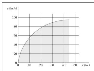
Shown in the figure is a portion of the experimentally determined v-x curve for a shuttle cart. Determine by approximate means the acceleration of the cart (a) when x = 10 in., (b) when v = 80 in./s.
