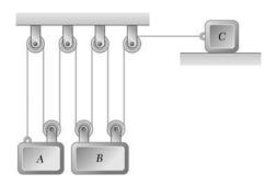
Block B starts from rest, block A moves with a constant acceleration, and slider block C moves to the right with a constant acceleration of 75 mm/s<sup>2</sup>. Knowing that at t = 2 s the velocities of B and C are 480 mm/s downward and 280 mm/s to the right, respectively, determine (a) the accelerations of A and B, (b) the initial velocities of A and C, (c) the change in position of slider block C after A s.
