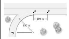
A motorist starts from rest at Point A on a circular entrance ramp when t = 0, increases the speed of her automobile at a constant rate and enters the highway at Point B. Knowing that her speed continues to increase at the same rate until it reaches 100 km/h at Point C, determine (a) the speed at Point B, (b) the magnitude of the total acceleration when t = 20 s.
