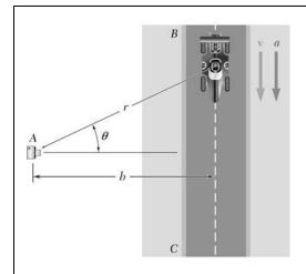
To study the performance of a racecar, a high-speed camera is positioned at Point A. The camera is mounted on a mechanism which permits it to record the motion of the car as the car travels on straightway BC. Determine (a) the speed of the car in terms of b,  $\theta$ , and  $\dot{\theta}$ , (b) the magnitude of the acceleration in terms of b,  $\theta$ , and  $\dot{\theta}$ .
