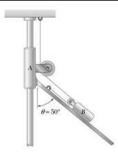
Knowing that at the instant shown assembly A has a velocity of 9 in./s and an acceleration of 15 in./s<sup>2</sup> both directed downward, determine (a) the velocity of block B, (b) the acceleration of block B.
