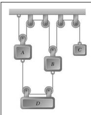
Block C starts from rest at t = 0 and moves downward with a constant acceleration of 4 in./s<sup>2</sup>. Knowing that block B has a constant velocity of 3 in./s upward, determine (a) the time when the velocity of block A is zero, (b) the time when the velocity of block A is equal to the velocity of block D, (c) the change in position of block A after S s.
