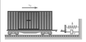
A loaded railroad car is rolling at a constant velocity when it couples with a spring and dashpot bumper system. After the coupling, the motion of the car is defined by the relation  $x = 60e^{-4.8t} \sin 16t$  where x and t are expressed in mm and seconds, respectively. Determine the position, the velocity and the acceleration of the railroad car when  $(a) \ t = 0$ ,  $(b) \ t = 0.3 \ s$ .
