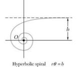
A particle moves along the spiral shown; determine the magnitude of the velocity of the particle in terms of b,  $\theta$ , and  $\dot{\theta}$ .
