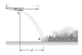
An airplane used to drop water on brushfires is flying horizontally in a straight line at 180 mi/h at an altitude of 300 ft. Determine the distance d at which the pilot should release the water so that it will hit the fire at B.
