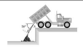
Coal is discharged from the tailgate A of a dump truck with an initial velocity  $\mathbf{v}_A = 2 \text{ m/s} > 50^\circ$ . Determine the radius of curvature of the trajectory described by the coal (a) at Point A, (b) at the point of the trajectory 1 m below Point A.
