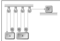
Block B moves downward with a constant velocity of 20 mm/s. At t = 0, block A is moving upward with a constant acceleration, and its velocity is 30 mm/s. Knowing that at t = 3 s slider block C has moved 57 mm to the right, determine (a) the velocity of slider block C at t = 0, (b) the accelerations of A and C, (c) the change in position of block A after 5 s.
