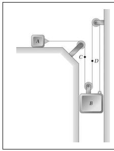
Block B starts from rest and moves downward with a constant acceleration. Knowing that after slider block A has moved 9 in. its velocity is 6 ft/s, determine (a) the accelerations of A and B, (b) the velocity and the change in position of B after 2 s.
