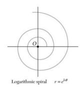
A particle moves along the spiral shown. Knowing that  $\dot{\theta}$  is constant and denoting this constant by  $\omega$ , determine the magnitude of the acceleration of the particle in terms of b,  $\theta$ , and  $\omega$ .
