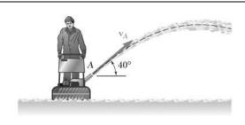
From a photograph of a homeowner using a snowblower, it is determined that the radius of curvature of the trajectory of the snow was 30 ft as the snow left the discharge chute at A. Determine (a) the discharge velocity  $\mathbf{v}_A$  of the snow, (b) the radius of curvature of the trajectory at its maximum height.
