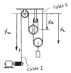
Let  $x_B$  and  $x_L$  be the positions, respectively, of pulley B and load L measured downward from a fixed elevation above both. Let  $x_M$  be the position of a point on the cable about to enter the reel driven by the motor. Then, considering the lengths of the two cables,
