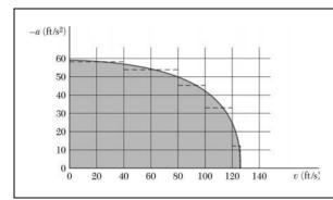
A training airplane has a velocity of 126 ft/s when it lands on an aircraft carrier. As the arresting gear of the carrier brings the airplane to rest, the velocity and the acceleration of the airplane are recorded; the results are shown (solid curve) in the figure. Determine by approximate means (a) the time required for the airplane to come to rest, (b) the distance traveled in that time.
