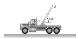
The end Point *B* of a boom is originally 5 m from fixed Point *A* when the driver starts to retract the boom with a constant radial acceleration of  $\ddot{r} = -1.0 \text{ m/s}^2$  and lower it with a constant angular acceleration  $\ddot{\theta} = -0.5 \text{ rad/s}^2$ . At t = 2 s, determine (a) the velocity of Point *B*, (b) the acceleration of Point *B*, (c) the radius of curvature of the path.
