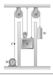
The elevator shown starts from rest and moves upward with a constant acceleration. If the counterweight W moves through 30 ft in 5 s, determine (a) the acceleration of the elevator and the cable C, (b) the velocity of the elevator after 5 s.
