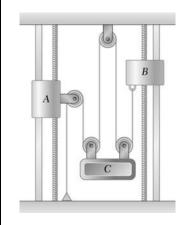
Collar A starts from rest at t = 0 and moves downward with a constant acceleration of 7 in./s<sup>2</sup>. Collar B moves upward with a constant acceleration, and its initial velocity is 8 in./s. Knowing that collar B moves through 20 in. between t = 0 and t = 2 s, determine (a) the accelerations of collar B and block C, (b) the time at which the velocity of block C is zero, (c) the distance through which block C will have moved at that time.
