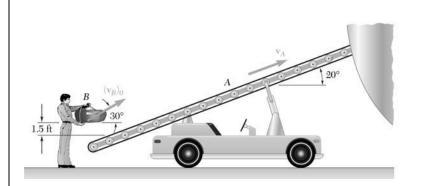
Conveyor belt A, which forms a  $20^{\circ}$  angle with the horizontal, moves at a constant speed of 4 ft/s and is used to load an airplane. Knowing that a worker tosses duffel bag B with an initial velocity of 2.5 ft/s at an angle of  $30^{\circ}$  with the horizontal, determine the velocity of the bag relative to the belt as it lands on the
