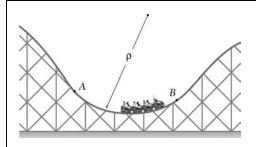
Determine the maximum speed that the cars of the roller-coaster can reach along the circular portion AB of the track if  $\rho$  is 25 m and the normal component of their acceleration cannot exceed 3 g.
