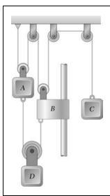
The system shown starts from rest, and each component moves with a constant acceleration. If the relative acceleration of block C with respect to collar B is  $60 \,\mathrm{mm/s^2}$  upward and the relative acceleration of block D with respect to block A is  $110 \,\mathrm{mm/s^2}$  downward, determine (a) the velocity of block C after 3 s, (b) the change in position of block D after 5 s.
