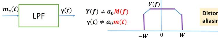
Distortion due to aliasing is observed
