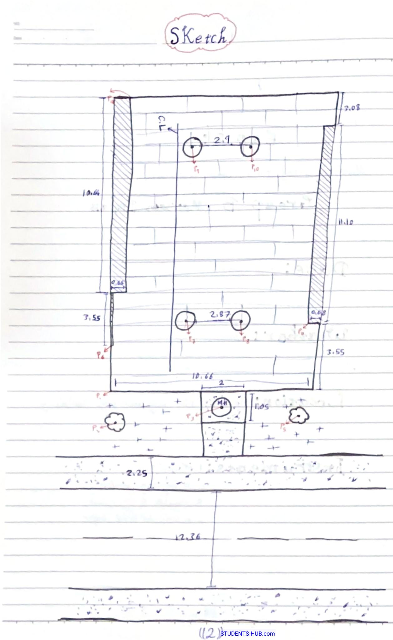
Ties Method Point d, d, d dy d, P, 3.4 15 12 5.3 P. 15 4 6.27 12 5,3 P, 12 15 2.94 P4 14 3.47 12 5.8 P. 15 6,57 7.72 13 Pé 12,7 12.59 Ρ, Pg 1.8 Pq-1.8 Pio 12.7 Pu
