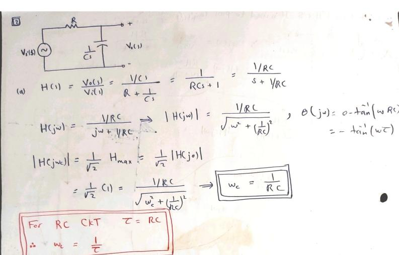
\* Choose values for Rg@ that will yield a low-pass filter with a cutoff frequency of 3 KHz.
