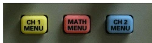
The **MATH MENU** button can be used to display an arithmetic combination of two signals. You can select from addition, subtraction, multiplication, addition or Fourier Transform (FFT). The resulting signal is plotted in red.
