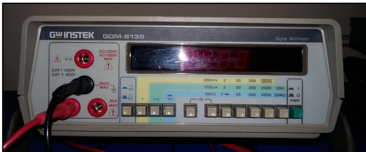
**Figure 2.3: Digital Multimeter GDM-8135, connected as ammeter.**
