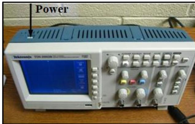
**Figure 2.11: Oscilloscope Tektronix TDS 2002B**
