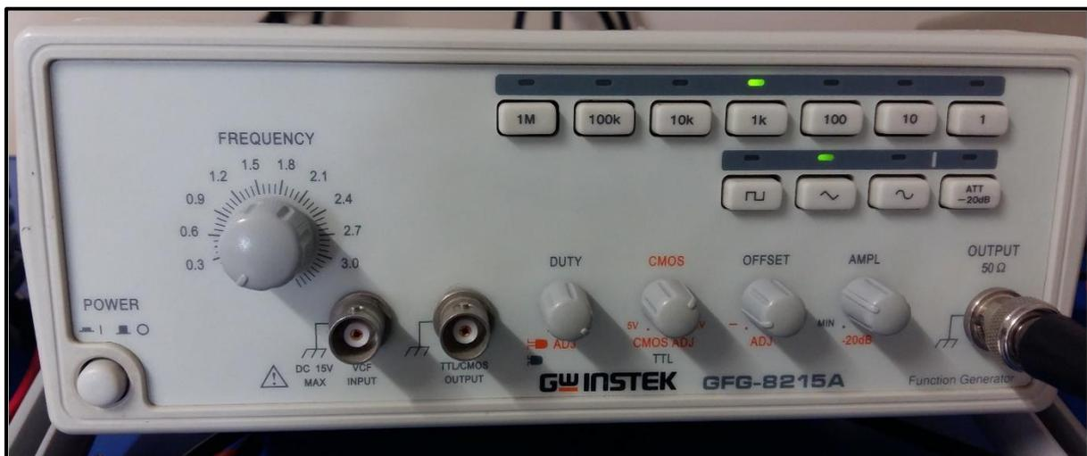
**Figure 2.10: Function Wave Generator GFG-8215a**
