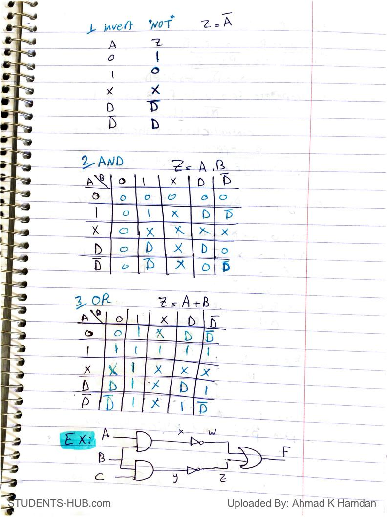
test B sal: put o on B -> B=D use path BXWF => A=1 X=D => W=D to propagate from w to f Z=0 ys1 BC=11 contradiction on the value of B -spath fails path ByZF will fail "symmetry" \* try path BXW F & BYZF together put o on B => B = D Asl -> X SD -> W SD -> F.D CSI -> YSD -> ZSD test vector ABC iffsI no fault 101 for faulty XX test B sap L path Bxf and BYZf together put 1 on D -> B=D A=1 - X=D C=1 - y=D -> Z=D
