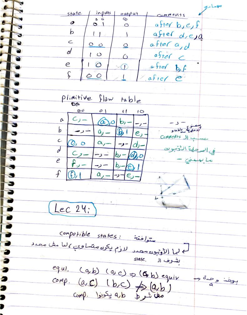
implication chart Compatible pairs: (a,b), (a,c), (a,d), (b,e), (b,f), (c,d), (e,f) maximal compatibles (merger diagram) (a, c,d) (b,e,f)(a,b) minimum set of maximal compatibles that covers all states and closed. لما كل ال ما في معهم نقر وكم بطع الع دوه (a, c, d) => covers all states & closed Uploaded By: Ahmad K Hamdan
