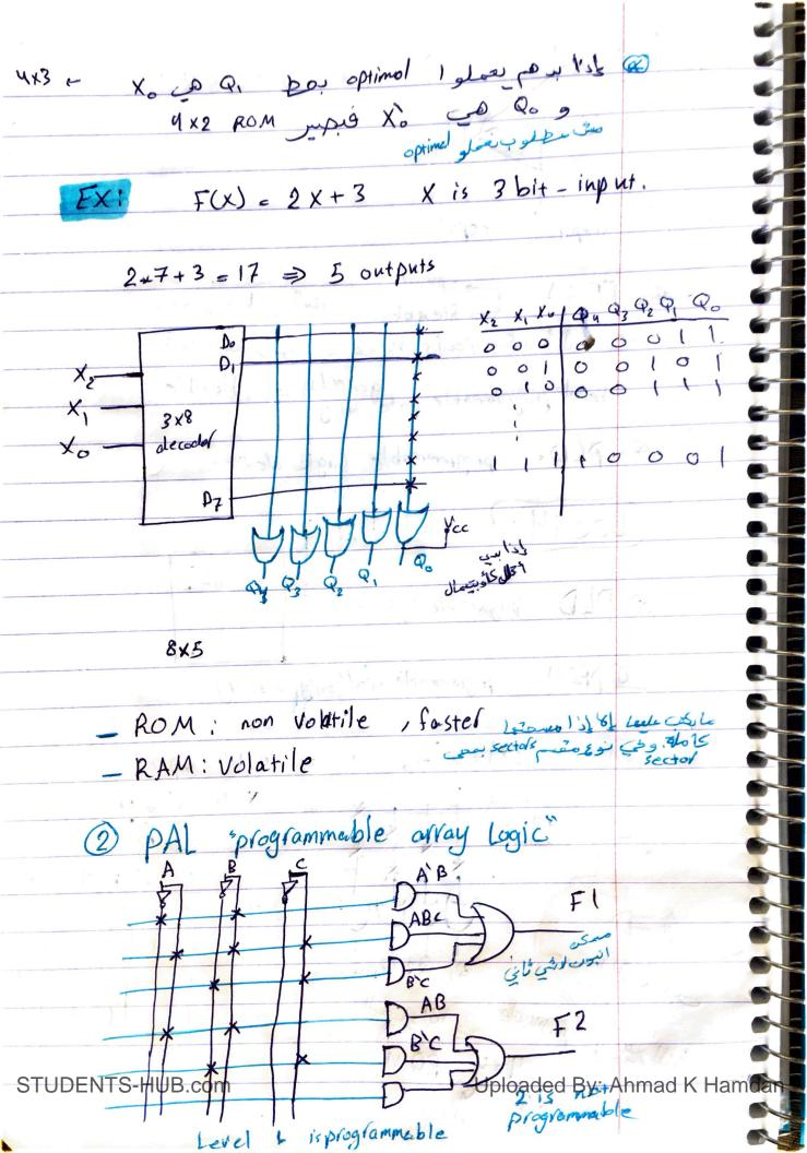
FI = A'B + ABC + B'C F1 = 2 F2 = AB + B'C aprogrammable Logic Array 7 7 7 7 7 ABC 5 2 levels are programmable s fis A'B+B'C+ABC f2 = B'C'+A'B FPGAs (Field programmable Gate Array) - FPGAs are usually based on book-up-table 7 LUT apploach. Ex: 2 input LUT will look like this mux 124 X1 tocations SRAM UXLS bit F=A and B 16 0 ino STUDENTS-HUB. Com Uploaded By Ahmad K Hamdan
