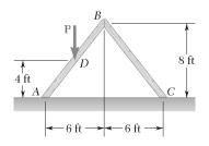
Two identical uniform boards, each of weight 40 lb, are temporarily leaned against each other as shown. Knowing that the coefficient of static friction between all surfaces is 0.40, determine (a) the largest magnitude of the force **P** for which equilibrium will be maintained, (b) the surface at which motion will impend.
