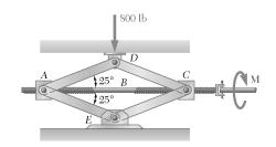
The position of the automobile jack shown is controlled by a screw ABC that is single-threaded at each end (right-handed thread at A, left-handed thread at C). Each thread has a pitch of 0.1 in. and a mean diameter of 0.375 in. If the coefficient of static friction is 0.15, determine the magnitude of the couple  $\mathbf{M}$  that must be applied to raise the automobile.
