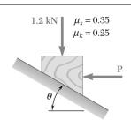
Determine whether the block shown is in equilibrium and find the magnitude and direction of the friction force when  $\theta = 30^{\circ}$  and P = 150 N.
