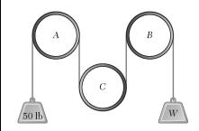
A cable is placed around three parallel pipes. Knowing that the coefficients of friction are  $\mu_s = 0.25$  and  $\mu_k = 0.20$ , determine (a) the smallest weight W for which equilibrium is maintained, (b) the largest weight W that can be raised if pipe B is slowly rotated counterclockwise while pipes A and C remain fixed.
