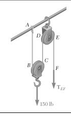
The block and tackle shown are used to lower a 150-lb load. Each of the 3-in-diameter pulleys rotates on a 0.5-in.-diameter axle. Knowing that the coefficient of static friction is 0.20, determine the tension in each portion of the rope as the load is slowly lowered.
