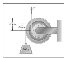
The double pulley shown is attached to a 10-mm-radius shaft that fits loosely in a fixed bearing. Knowing that the coefficient of static friction between the shaft and the poorly lubricated bearing is 0.40, determine the magnitude of the force **P** required to start raising the load.
