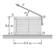
A 40-kg packing crate must be moved to the left along the floor without tipping. Knowing that the coefficient of static friction between the crate and the floor is 0.35, determine (a) the largest allowable value of  $\alpha$ , (b) the corresponding magnitude of the force **P**.
