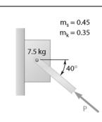
Draw the free-body diagram needed to determine the smallest force  ${\bf P}$  for which equilibrium of the 7.5-kg block is maintained.
