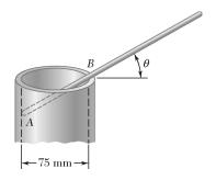
A slender steel rod of length 225 mm is placed inside a pipe as shown. Knowing that the coefficient of static friction between the rod and the pipe is 0.20, determine the largest value of  $\theta$  for which the rod will not fall into the pipe.
