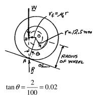
Since a scooter rolls at constant speed, each wheel is in <u>equilibrium</u>. Thus, **W** and **R** must have a <u>common line</u> of action tangent to the friction circle.
