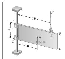
The 50-lb plate ABCD is attached at A and D to collars that can slide on the vertical rod. Knowing that the coefficient of static friction is 0.40 between both collars and the rod, determine whether the plate is in equilibrium in the position shown when the magnitude of the vertical force applied at E is (a) P = 0, (b) P = 20 lb.
