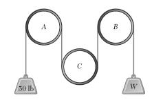
A cable is placed around three parallel pipes. Two of the pipes are fixed and do not rotate; the third pipe is slowly rotated. Knowing that the coefficients of friction are  $\mu_s = 0.25$  and  $\mu_k = 0.20$ , determine the largest weight W that can be raised (a) if only pipe Ais rotated counterclockwise, (b) if only pipe C is rotated clockwise.
