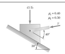
Determine whether the block shown is in equilibrium and find the magnitude and direction of the friction force when P = 100 lb.
