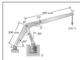
The press shown is used to emboss a small seal at E. Knowing that the coefficient of static friction between the vertical guide and the embossing die D is 0.30, determine the force exerted by the die on the seal.
