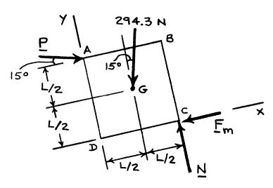
For impending tip, **N** must act at *C*. For impending slip,
