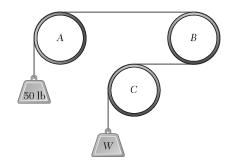
A cable is placed around three parallel pipes. Two of the pipes are fixed and do not rotate; the third pipe is slowly rotated. Knowing that the coefficients of friction are  $\mu_s = 0.25$  and  $\mu_k = 0.20$ , determine the largest weight W that can be raised (a) if only pipe Ais rotated counterclockwise, (b) if only pipe C is rotated clockwise.
