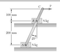
Two 8-kg blocks A and B resting on shelves are connected by a rod of negligible mass. Knowing that the magnitude of a horizontal force P applied at C is slowly increased from zero, determine the value of P for which motion occurs, and what that motion is, when the coefficient of static friction between all surfaces is (a)  $\mu_s = 0.40$ , (b)  $\mu_s = 0.50$ .
