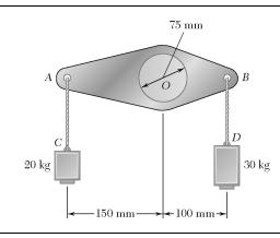
A lever of negligible weight is loosely fitted onto a 75-mm-diameter fixed shaft. It is observed that the lever will just start rotating if a 3-kg mass is added at *C*. Determine the coefficient of static friction between the shaft and the lever.
