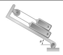
The 20-lb block A and the 30-lb block B are supported by an incline that is held in the position shown. Knowing that the coefficient of static friction is 0.15 between the two blocks and zero between block B and the incline, determine the value of  $\theta$  for which motion is impending.
