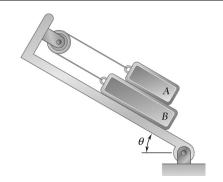
The 20-lb block A and the 30-lb block B are supported by an incline that is held in the position shown. Knowing that the coefficient of static friction is 0.15 between all surfaces of contact, determine the value of  $\theta$  for which motion is impending.
