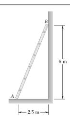
A 6.5-m ladder AB leans against a wall as shown. Assuming that the coefficient of static friction  $\mu_s$  is zero at B, determine the smallest value of  $\mu_s$  at A for which equilibrium is maintained.
