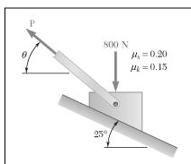
Determine whether the block shown is in equilibrium and find the magnitude and direction of the friction force when  $\theta = 35^{\circ}$  and P = 200 N.
