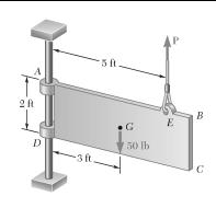
In Problem 8.29, determine the range of values of the magnitude *P* of the vertical force applied at *E* for which the plate will move downward.
