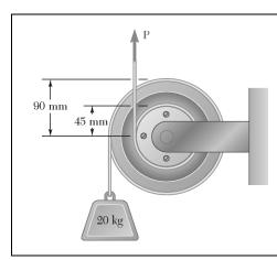
The double pulley shown is attached to a 10-mm-radius shaft that fits loosely in a fixed bearing. Knowing that the coefficient of static friction between the shaft and the poorly lubricated bearing is 0.40, determine the magnitude of the smallest force  $\bf P$  required to maintain equilibrium.
