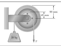
The double pulley shown is attached to a 10-mm-radius shaft that fits loosely in a fixed bearing. Knowing that the coefficient of static friction between the shaft and the poorly lubricated bearing is 0.40, determine the magnitude of the force **P** required to start raising the load.
