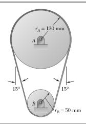
A flat belt is used to transmit a couple from drum B to drum A. Knowing that the coefficient of static friction is 0.40 and that the allowable belt tension is 450 N, determine the largest couple that can be exerted on drum A.
