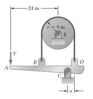
The speed of the brake drum shown is controlled by a belt attached to the control bar AD. Knowing that a=4 in., determine the maximum value of the coefficient of static friction for which the brake is not self-locking when the drum rotates counterclockwise.
