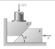
Block A supports a pipe column and rests as shown on wedge B. Knowing that the coefficient of static friction at all surfaces of contact is 0.25 and that  $\theta = 45^{\circ}$ , determine the smallest force **P** for which equilibrium is maintained.
