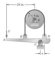
The speed of the brake drum shown is controlled by a belt attached to the control bar AD. A force **P** of magnitude 25 lb is applied to the control bar at A. Determine the magnitude of the couple being applied to the drum, knowing that the coefficient of kinetic friction between the belt and the drum is 0.25, that a = 4 in., and that the drum is rotating at a constant speed (a) counterclockwise, (b) clockwise.
