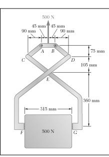
A 500-N concrete block is to be lifted by the pair of tongs shown. Determine the smallest allowable value of the coefficient of static friction between the block and the tongs at F and G.
