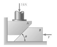
Block A supports a pipe column and rests as shown on wedge B. Knowing that the coefficient of static friction at all surfaces of contact is 0.25 and that  $\theta = 45^{\circ}$ , determine the smallest force **P** required to raise block A.
