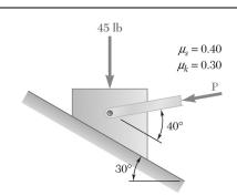
Determine the smallest value of P required to (a) start the block up the incline, (b) keep it moving up, (c) prevent it from moving down.
