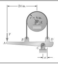
The speed of the brake drum shown is controlled by a belt attached to the control bar AD. Knowing that the coefficient of static friction is 0.30 and that the brake drum is rotating counterclockwise, determine the minimum value of a for which the brake is not self-locking.
