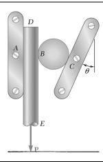
A rod DE and a small cylinder are placed between two guides as shown. The rod is not to slip downward, however large the force **P** may be; i.e., the arrangement is said to be self-locking. Neglecting the weight of the cylinder, determine the minimum allowable coefficients of static friction at A, B, and C.
