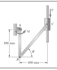
Knowing that the coefficient of static friction between the collar and the rod is 0.35, determine the range of values of P for which equilibrium is maintained when  $\theta = 50^{\circ}$  and  $M = 20 \text{ N} \cdot \text{m}$ .
