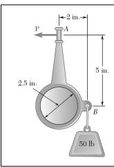
A lever AB of negligible weight is loosely fitted onto a 2.5-in.-diameter fixed shaft. Knowing that the coefficient of static friction between the fixed shaft and the lever is 0.15, determine the force  $\mathbf{P}$  required to start the lever rotating clockwise.
