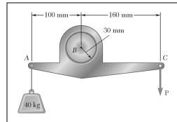
A lever of negligible weight is loosely fitted onto a 30-mm-radius fixed shaft as shown. Knowing that a force **P** of magnitude 275 N will just start the lever rotating clockwise, determine (a) the coefficient of static friction between the shaft and the lever, (b) the smallest force **P** for which the lever does not start rotating counterclockwise.
