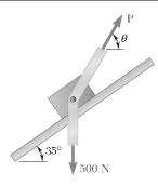
The coefficients of friction between the block and the rail are  $\mu_s = 0.30$  and  $\mu_k = 0.25$ . Knowing that  $\theta = 65^\circ$ , determine the smallest value of *P* required (a) to start the block moving up the rail, (b) to keep it from moving down.
