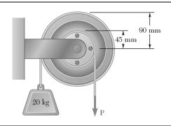
The double pulley shown is attached to a 10-mm-radius shaft that fits loosely in a fixed bearing. Knowing that the coefficient of static friction between the shaft and the poorly lubricated bearing is 0.40, determine the magnitude of the smallest force  $\bf P$  required to maintain equilibrium.
