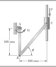
Knowing that the coefficient of static friction between the collar and the rod is 0.40, determine the range of values of M for which equilibrium is maintained when  $\theta = 60^{\circ}$  and P = 200 N.
