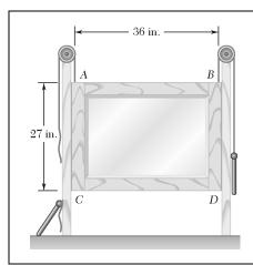
A window sash weighing 10 lb is normally supported by two 5-lb sash weights. Knowing that the window remains open after one sash cord has broken, determine the smallest possible value of the coefficient of static friction. (Assume that the sash is slightly smaller than the frame and will bind only at Points A and D.)
