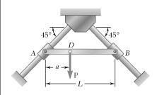
Bar AB is attached to collars that can slide on the inclined rods shown. A force **P** is applied at Point D located at a distance a from end A. Knowing that the coefficient of static friction  $\mu_s$  between each collar and the rod upon which it slides is 0.30 and neglecting the weights of the bar and of the collars, determine the smallest value of the ratio a/L for which equilibrium is maintained.
