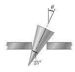
A conical wedge is placed between two horizontal plates that are then slowly moved toward each other. Indicate what will happen to the wedge (a) if  $\mu_s = 0.20$ , (b) if  $\mu_s = 0.30$ .
