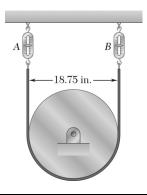
The setup shown is used to measure the output of a small turbine. The coefficient of kinetic friction is 0.20 and the reading of each spring scale is 16 lb when the flywheel is at rest. Determine (a) the reading of each scale when the flywheel is rotating clockwise at a constant speed, (b) the couple that must be applied to the flywheel. Assume that the length of the belt does not change.
