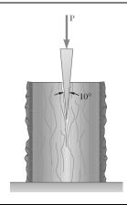
A  $10^{\circ}$  wedge is used to split a section of a log. The coefficient of static friction between the wedge and the log is 0.35. Knowing that a force **P** of magnitude 600 lb was required to insert the wedge, determine the magnitude of the forces exerted on the wood by the wedge after insertion.
