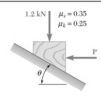
Determine whether the block shown is in equilibrium and find the magnitude and direction of the friction force when  $\theta = 25^{\circ}$  and P = 750 N.
