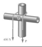
Knowing that the coefficient of static friction is 0.30 between the rope and the horizontal pipe and that the smallest value of P for which equilibrium is maintained is 80 N, determine (a) the largest value of P for which equilibrium is maintained, (b) the coefficient of static friction between the rope and the vertical pipe.
