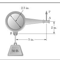
A lever AB of negligible weight is loosely fitted onto a 2.5-in.-diameter fixed shaft. Knowing that the coefficient of static friction between the fixed shaft and the lever is 0.15, determine the force  $\bf P$  required to start the lever rotating counterclockwise.
