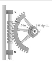
The square-threaded worm gear shown has a mean radius of 2 in. and a lead of 0.5 in. The large gear is subjected to a constant clockwise couple of 9.6 kip  $\cdot$  in. Knowing that the coefficient of static friction between the two gears is 0.12, determine the couple that must be applied to shaft AB in order to rotate the large gear counterclockwise. Neglect friction in the bearings at A, B, and C.
