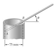
In Problem 8.44, determine the smallest value of  $\theta$  for which the rod will not fall out the pipe.
