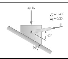
Determine whether the block shown is in equilibrium and find the magnitude and direction of the friction force when P = 60 lb.
