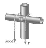
Knowing that the coefficient of static friction is 0.25 between the rope and the horizontal pipe and 0.20 between the rope and the vertical pipe, determine the range of values of P for which equilibrium is maintained.
