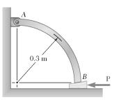
A  $10^{\circ}$  wedge is to be forced under end B of the 5-kg rod AB. Knowing that the coefficient of static friction is 0.40 between the wedge and the rod and 0.20 between the wedge and the floor, determine the smallest force **P** required to raise end B of the rod.
