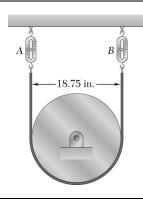
The setup shown is used to measure the output of a small turbine. When the flywheel is at rest, the reading of each spring scale is 14 lb. If a 105-lb  $\cdot$  in. couple must be applied to the flywheel to keep it rotating clockwise at a constant speed, determine (a) the reading of each scale at that time, (b) the coefficient of kinetic friction. Assume that the length of the belt does not change.
