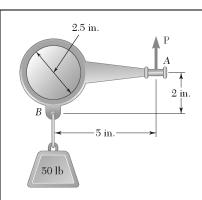
A lever AB of negligible weight is loosely fitted onto a 2.5-in.-diameter fixed shaft. Knowing that the coefficient of static friction between the fixed shaft and the lever is 0.15, determine the force  $\bf P$  required to start the lever rotating clockwise.
