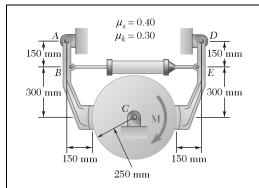
The hydraulic cylinder shown exerts a force of 3 kN directed to the right on Point B and to the left on Point E. Determine the magnitude of the couple M required to rotate the drum clockwise at a constant speed.
