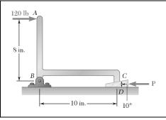
The machine part ABC is supported by a frictionless hinge at B and a  $10^{\circ}$  wedge at C. Knowing that the coefficient of static friction is 0.20 at both surfaces of the wedge, determine (a) the force P required to move the wedge to the left, (b) the components of the corresponding reaction at B.
