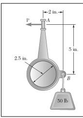
A lever AB of negligible weight is loosely fitted onto a 2.5-in.-diameter fixed shaft. Knowing that the coefficient of static friction between the fixed shaft and the lever is 0.15, determine the force  $\bf P$  required to start the lever rotating counterclockwise.
