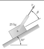
Knowing that the coefficient of friction between the 25-kg block and the incline is  $\mu_s = 0.25$ , determine (a) the smallest value of P required to start the block moving up the incline, (b) the corresponding value of  $\beta$ .
