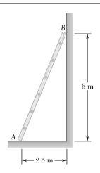
A 6.5-m ladder AB leans against a wall as shown. Assuming that the coefficient of static friction  $\mu_s$  is the same at A and B, determine the smallest value of  $\mu_s$  for which equilibrium is maintained.
