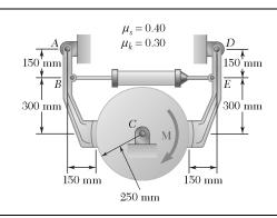
A couple **M** of magnitude  $100 \text{ N} \cdot \text{m}$  is applied to the drum as shown. Determine the smallest force that must be exerted by the hydraulic cylinder on joints B and E if the drum is not to rotate.
