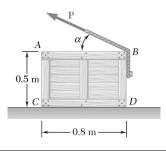
A 40-kg packing crate is pulled by a rope as shown. The coefficient of static friction between the crate and the floor is 0.35. If  $\alpha = 40^{\circ}$ , determine (a) the magnitude of the force **P** required to move the crate, (b) whether the crate will slide or tip.
