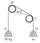
A rope ABCD is looped over two pipes as shown. Knowing that the coefficient of static friction is 0.25, determine (a) the smallest value of the mass m for which equilibrium is possible, (b) the corresponding tension in portion BC of the rope.
