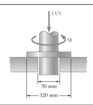
Knowing that a couple of magnitude  $30~N\cdot m$  is required to start the vertical shaft rotating, determine the coefficient of static friction between the annular surfaces of contact.
