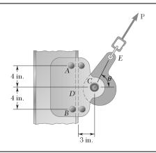
To be of practical use, the safety sleeve described in Problem 8.34 must be free to slide along the rail when pulled upward. Determine the largest allowable value of the coefficient of static friction between the flange of the rail and the pins at A and B if the sleeve is to be free to slide when pulled as shown in the figure, assuming (a)  $\theta = 60^{\circ}$ , (b)  $\theta = 50^{\circ}$ , (c)  $\theta = 40^{\circ}$ .
