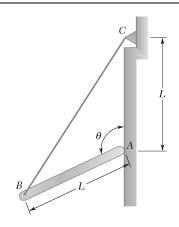
End A of a slender, uniform rod of length L and weight W bears on a surface as shown, while end B is supported by a cord BC. Knowing that the coefficients of friction are  $\mu_s = 0.40$  and  $\mu_k = 0.30$ , determine (a) the largest value of  $\theta$  for which motion is impending, (b) the corresponding value of the tension in the cord.
