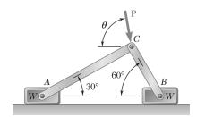
Two slender rods of negligible weight are pin-connected at C and attached to blocks A and B, each of weight W. Knowing that P = 1.260W and that the coefficient of static friction between the blocks and the horizontal surface is 0.30, determine the range of values of  $\theta$ , between 0 and 180°, for which equilibrium is maintained.
