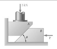
Block A supports a pipe column and rests as shown on wedge B. The coefficient of static friction at all surfaces of contact is 0.25. If P = 0, determine (a) the angle  $\theta$  for which sliding is impending, (b) the corresponding force exerted on the block by the vertical wall.
