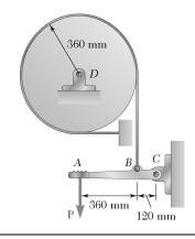
A band brake is used to control the speed of a flywheel as shown. The coefficients of friction are  $\mu_s = 0.30$  and  $\mu_k = 0.25$ . Determine the magnitude of the couple being applied to the flywheel, knowing that P = 45 N and that the flywheel is rotating counterclockwise at a constant speed.
