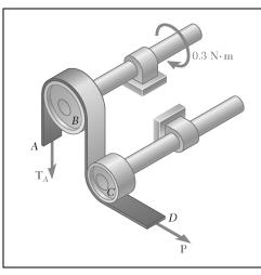
A recording tape passes over the 20-mm-radius drive drum B and under the idler drum C. Knowing that the coefficients of friction between the tape and the drums are  $\mu_s = 0.40$  and  $\mu_k = 0.30$  and that drum C is free to rotate, determine the smallest allowable value of P if slipping of the tape on drum B is not to occur.
