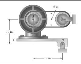
In the pivoted motor mount shown the weight W of the 175-lb motor is used to maintain tension in the drive belt. Knowing that the coefficient of static friction between the flat belt and drums A and B is 0.40, and neglecting the weight of platform CD, determine the largest couple that can be transmitted to drum B when the drive drum A is rotating clockwise.
