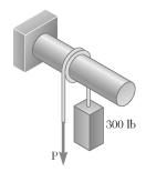
A 300-lb block is supported by a rope that is wrapped  $1\frac{1}{2}$  times around a horizontal rod. Knowing that the coefficient of static friction between the rope and the rod is 0.15, determine the range of values of P for which equilibrium is maintained.
