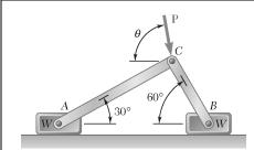
Two slender rods of negligible weight are pin-connected at C and attached to blocks A and B, each of weight W. Knowing that  $\theta = 80^{\circ}$  and that the coefficient of static friction between the blocks and the horizontal surface is 0.30, determine the largest value of P for which equilibrium is maintained.
