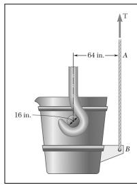
A hot-metal ladle and its contents weigh 130 kips. Knowing that the coefficient of static friction between the hooks and the pinion is 0.30, determine the tension in cable AB required to start tipping the ladle.
