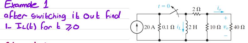
Step 1 :find I(0-), from the Circuit directly or on the Jaw Since we have a Curret source => IL(0-) = 20 A
