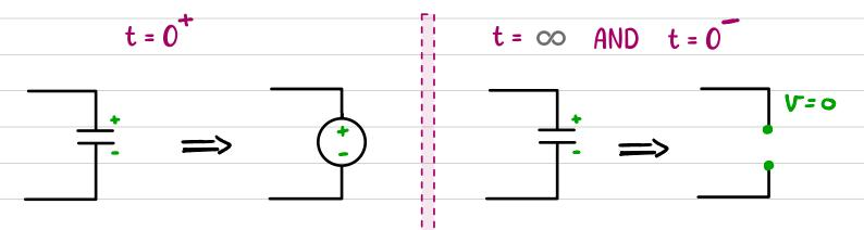
\* At  $t = 0^+$  the Cafacitor \* At  $t = \infty$  And  $t = 0^-$ , the Can be considered as a Cafacitor Can be considered Voltage Source. as a open Circuit
