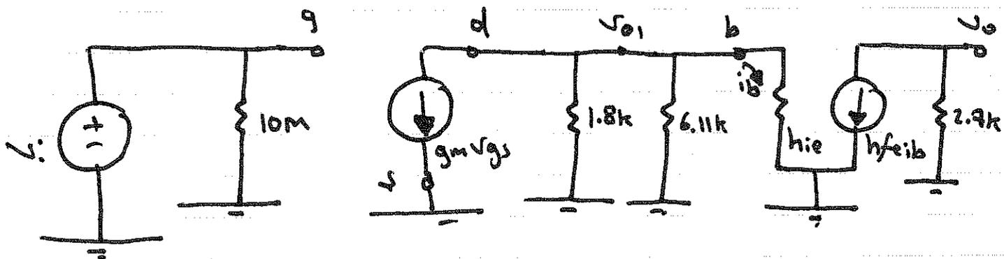
$$A_{v1} = \frac{V_{01}}{V_i} ; V_{01} = -g_m V_{gs} (1.8k \parallel 6.11k \parallel h_{ie})$$
