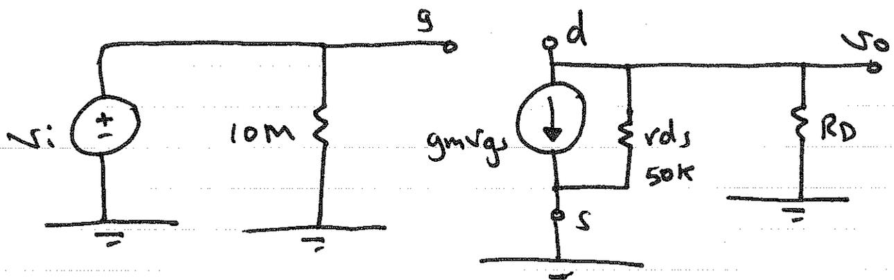
$$V_o = -g_m V_{gs} (50 \text{ K} \parallel R_D)$$
