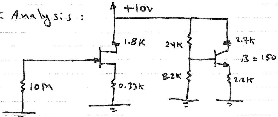
$$I_{DSS} = 6 \text{ mA} , V_p = -3 \text{ V}$$
