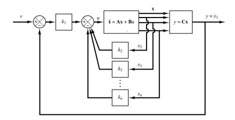
the reference input r is a step function. In this system we use the following state-feedback control scheme:
