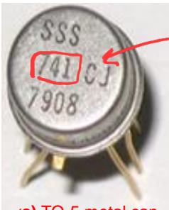
(c) TO-5 metal can 8-Leads package
