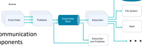
asynchronous communication style where components communicate through the production (Publisher) and consumption (Subscriber) of events.
