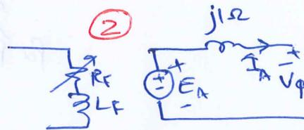
c)  $\bar{E}_A = \bar{V}_\phi + jX_s \bar{I}_A$
