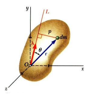
•  $I_{OL}$  = moment of inertia with respect to axis OL
