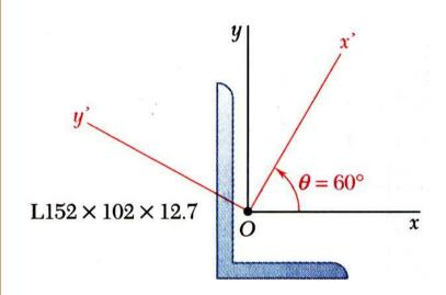
The moments and product of inertia with respect to the x and y axes are  $I_x = 7.24 \times 106 \text{ mm}^4$ ,  $I_y = 2.61 \times 106 \text{ mm}^4$ , and  $I_{xy} = -2.54 \times 10^6 \text{ mm}^4$ .
