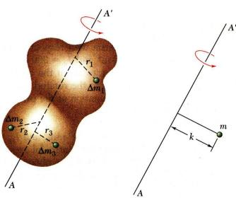
• Angular acceleration about the axis AA of the small mass  $\Delta m$  due to the application of a couple is proportional to  $r^2\Delta m$ .
