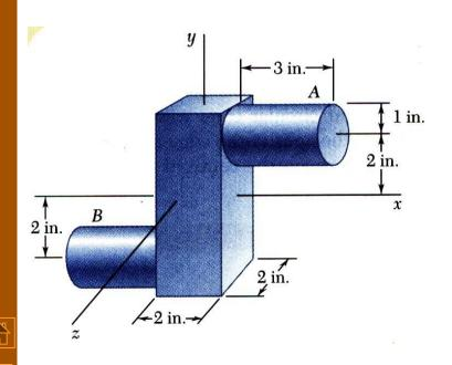
Determine the moments of inertia of the steel forging with respect to the *xyz* coordinate axes, knowing that the specific weight of steel is 490 lb/ft3.
