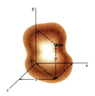
• Moment of inertia with respect to the *y* coordinate axis is
