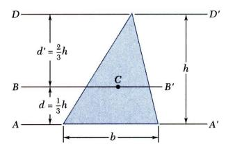
• Moment of inertia of a triangle with respect to a centroidal axis,
