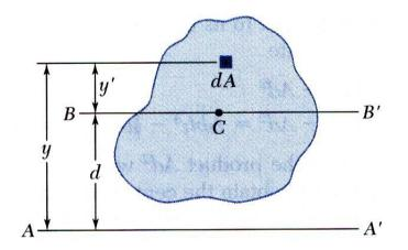
• Consider moment of inertia *I* of an area *A* with respect to the axis *AA*'
