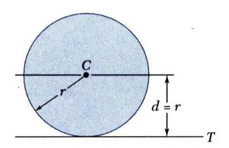
• Moment of inertia  $I_T$  of a circular area with respect to a tangent to the circle,
