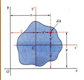
• Parallel axis theorem for products of inertia:
