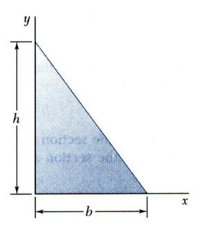
Determine the product of inertia of the right triangle (a) with respect to the x and y axes and (b) with respect to centroidal axes parallel to the x and y axes.
