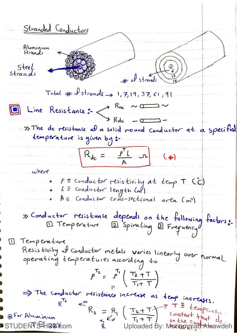
Since a stranded conductor is spiraled, each strand is longer than the finished conductor. This results in a slightly higher resistance than the value Calculated using equalish (\*)
