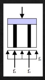
$P = f_c (A_g + (n - 1)A_s)$ Where: f<sub>c</sub> is stress in *concrete*  $f_s =$
