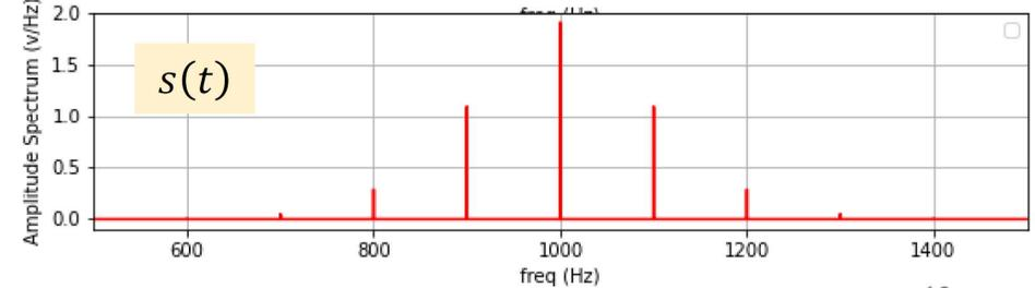
$BW = (f_c + 2f_m) - (f_c - 2f_m) = 4f_m = 400 \text{ Hz}$
