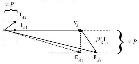
Since the power supplied by the motor is constant, the quantity  $I_A \cos \theta$ , which is directly proportional to power, must be constant. Therefore,
