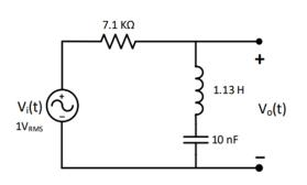
output voltage was observed to be nearly the same as the input voltage, indicating maximum output. As the frequency increased, the output voltage gradually decreased, reaching nearly zero at the center frequency. After passing the center frequency, the output voltage began to rise again, reaching a maximum at the cutoff frequencies fc1 and fc2, which were measured using the formula Vmax/ sqrt 2. These measurements were taken using both an oscilloscope and a digital multimeter.
