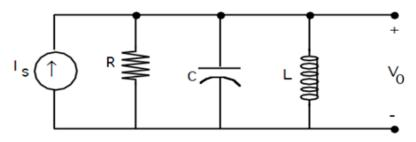
However, the resonant frequency for both circuit types converges to the same expression when the circuit's resistance is small. In a parallel RLC circuit, one way to define the resonant frequency is as the frequency at which the circuit's impedance is at its maximum.
