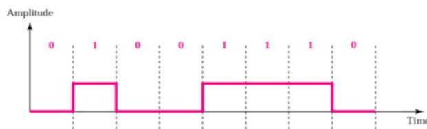
Unipolar Non-Return to Zero Signal
