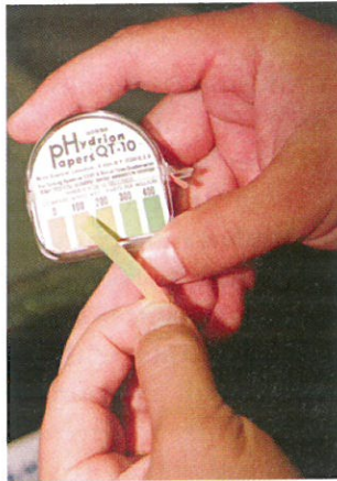
Figure 7.12 Measuring the Concentration of Sanitizers Using Test Strips
