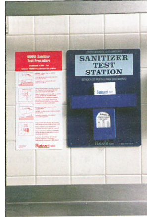
Figure 7.12 Measuring the Concentration of Sanitizers Using Test Strips
