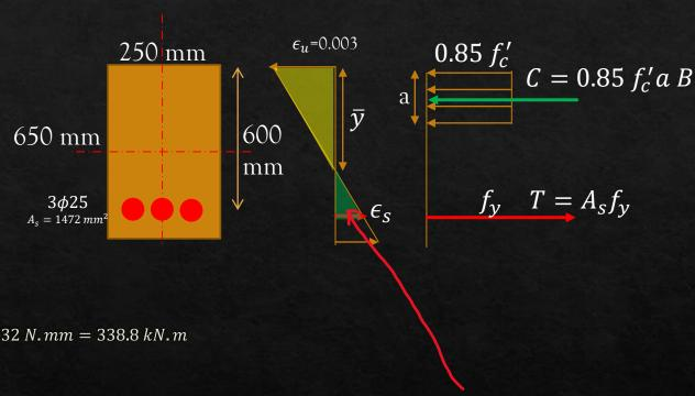
At failure, the strain in concrete is  $\epsilon_u$ = 0.003: the corresponding strain in steel at failure can be found by comparing the two triangles shown
