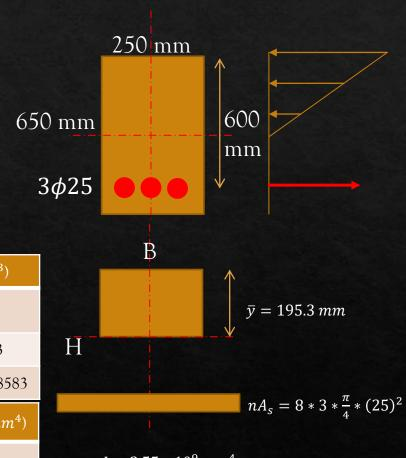
♦ Phase 2: Linear cracked section  $(M > M_{cr})$
